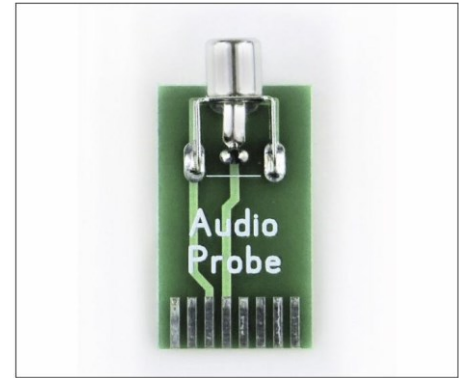
Figure 9: Adapter board for the AF probe
